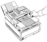
2. Neatly stack your documents, and then insert them face down into the document feeder. If necessary, readjust the document guides for a snug fit.
